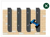
Always pre drill the wood plastic composite cladding using a minimum of a 4.5mm drill bit. If you do not you risk damaging the product over time.
