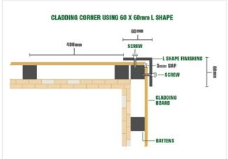
SCREW HOLES HAVE TO BE PRE DRILLED
