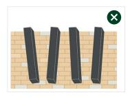
Batten must be laid on a solid flat surface such as a brick wall. Without this it will cause movement and be potentially dangerous.
