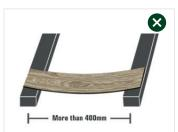
Battens must be set to a minimum of 400mm centres. If not boards may warp or move uncontrollably. Composite battens need to be fully supported along their length.
