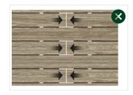
Butted boards must have 3mm gap. If not boards may warp or crack under pressure.
