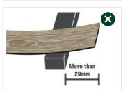
Ends of cladding boards panels must be supported and not have an overhang of more than 20mm. If not boards will move or be damaged.
